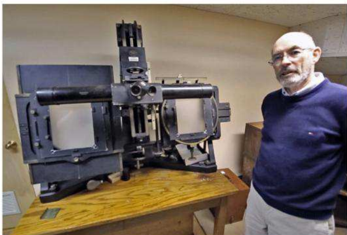
This blink comparator dates to 1905. Astronomers at Yerkes used it to discover high proper motion stars, variable stars, and other changing celestial phenomena.
