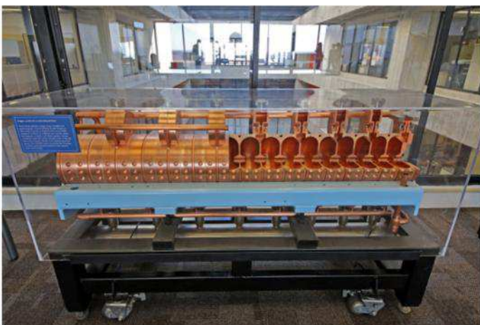
This copper cavity accelerates particles to high energy. A beam of particles enters and travels in sync with an 805-megahertz wave, gaining speed and energy. Fermilab has 30 strings of such cavities that can accelerate protons to three-quarters the speed of light. MICHAEL E. BAKICH
